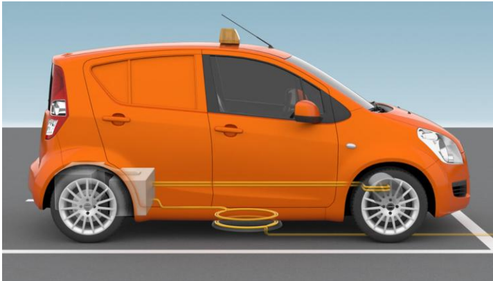
Caption: Inductive charging over an air gap beneath the car underbody
