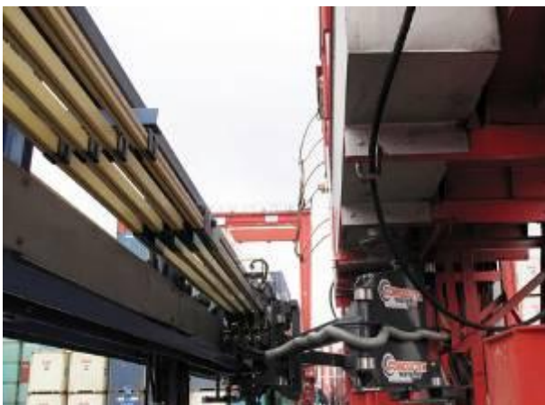
Caption: Electrification solutions of Conductix-Wampfler help to considerably reduce diesel consumption, CO2-emission and energy costs of container cranes
